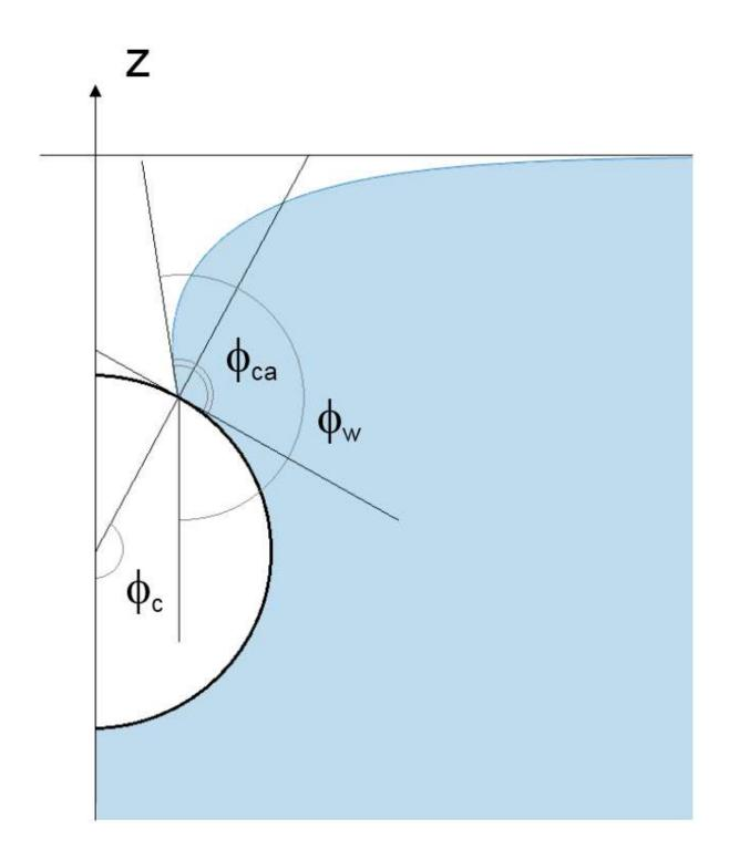
Fig. 3 Cylindrical body (just one half is shown) submerged in water (shown in blue). Undisturbed water level is at z=0,  $\phi_{ca}$  is the water contact angle,  $\phi_{c}$  is the angle between z-axis and a line going through the center of cylinder and the point of the water meniscus contact on the cylinder,  $\phi_{w}$  the angle between water meniscus surface and a vertical.
