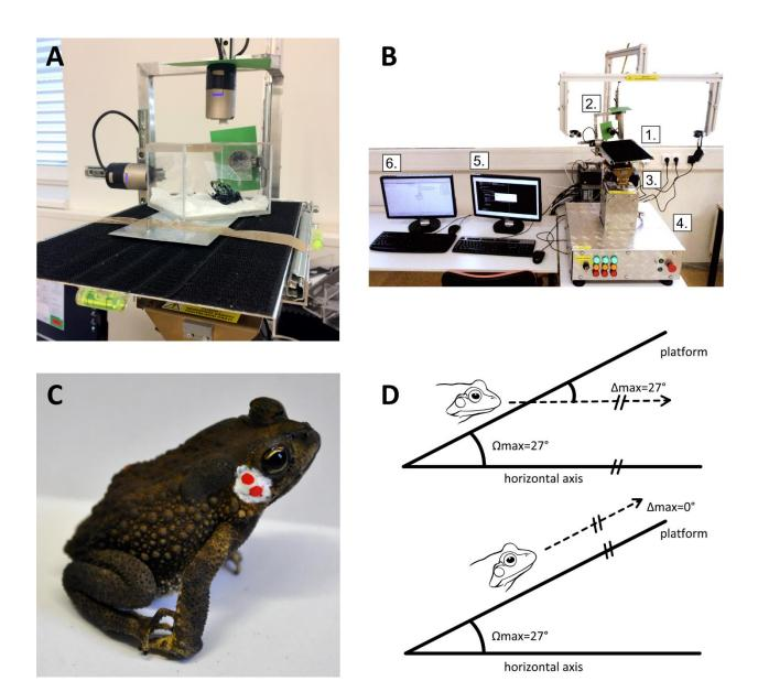
**Figure 1. Experimental design scheme.** The detail of frog in experimental box (A), the laboratory system measuring animal body response on a dynamic platform (B), the detail of frog's head with
