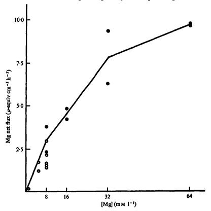
Fig. 4. The concentration-velocity curve for magnesium transport from the direct measurement of the <sup>38</sup>Mg net flux in Table 1 (open circles) and from the indirect measurement by the depression of the  $I_{so}$  as in Fig. 2 (closed circles). The line connects the midpoints of the depression of the  $I_{so}$  from two separate experiments.
