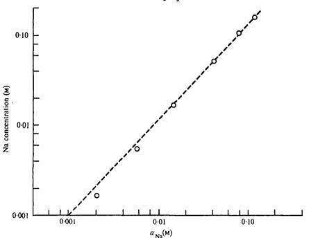
Fig. 1. The relation between sodium activity  $(a_{Na})$  and concentration. The line shows the theoretical relation calculated for pure NaCl solutions from the data of Robinson & Stokes (1959). The points indicate the values of  $a_{Na}$  measured with the sodium-selective electrode in physiological saline.
