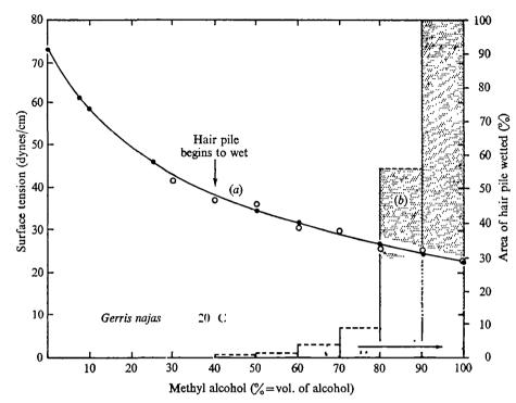
Fig. 1. (a) Curve showing the relationship between the surface tension and concentration of pure methyl alcohol in water. Closed circles from data supplied by Weast (1969), open circles from determinations by a simple capillary method. (b) Histogram showing the effect of immersion in graded solutions of methyl alcohol in water on the area of abdominal hair pile wetted. Mean values from determinations on six adults.
