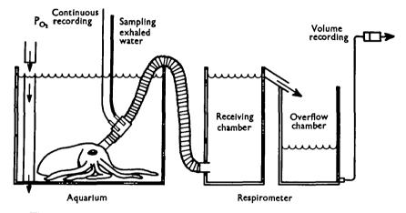
Fig. 1. The animal connected to the respirometer. The receiving chamber is connected to the octopus via a flexible hose. A plastic holder for mounting the polarographic oxygen electrodes and tubes for water sampling are shunted into the connecting hose. The overflow chamber receives the expired water, whose volume is recorded continuously.
