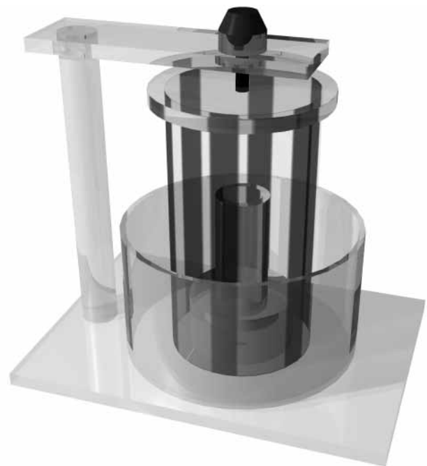
Fig. 1. The apparatus used to elicit an optomotor response in the tadpoles. A motor rotates the spindle at the top. This, in turn, rotates the striped cylinder around the vial which contains the tadpole.
