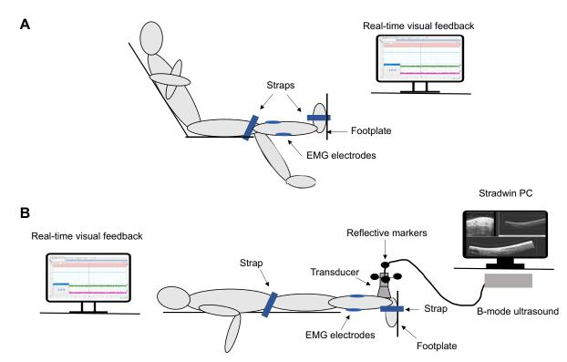
Fig. 1. Schematic diagram of the experimental setup. (A) Setup during the interventions. (B) Setup during the maximal voluntary isometric contraction (MVIC) tests and freehand 3D scanning. The interventions were performed with the participant in a sitting position to avoid any discomfort associated with a prolonged prone position.
