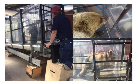
Fig. 1. The treadmill and its modifications used to measure energy expenditure of grizzly bears while lying, sitting, standing and walking on horizontal and up and down slopes. Both up and down slopes were created by lifting the front or back of the treadmill to the desired angle, and bears were encouraged to walk at a specific speed by providing small food rewards (e.g. apple slices).
