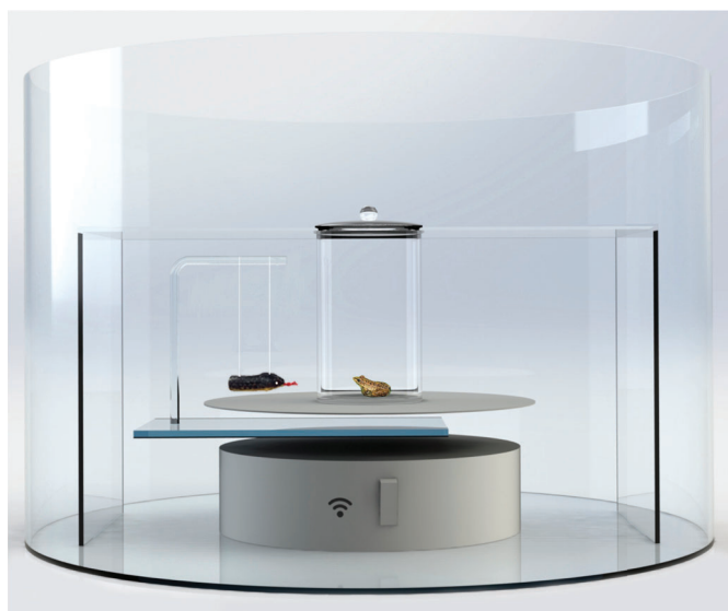
Fig. 2. The testing apparatus for behavioral and EEG experiments on N. daunchina . The subject was placed in a cylindrical cup made of transparent polymethyl methacrylate (PMMA), which was hung in the middle of a U-shaped frame. A bar made of transparent PMMA was bent to form a right angle and adhered onto a PMMA board placed on the electric turntable. A white plastic wafer was adhered to the bottom of the cup to try to avoid visual interference. In addition, a white opaque plastic cylinder surrounded all the components.
