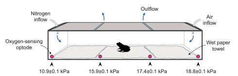
Fig. 1. Schematic representation of a custom-built experimental choice chamber. The partial pressure of O $_2$  ( $P_{O_2}$ ) range within the low O $_2$  zone (left), medium O $_2$  zone (centre) and high O $_2$  zone (right) was determined using O $_2$ -sensing optodes and a Presens Optical Oxygen Sensor. The choice chambers used for Cyclorana alboguttata were 750×240×120 mm and made from clear acrylic.
