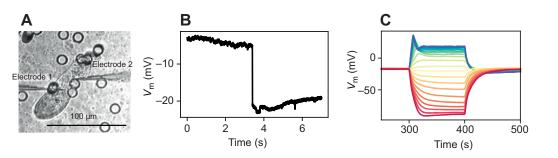
Fig. 2. Electrophysiology experiments on immobilized *Paramecium*. (A) Immobilized *Paramecium* impaled by two microelectrodes. (B) Membrane potential  $(V_m)$  measured while the electrode is impaled into the cell. Successful impalement is signalled by a sudden voltage drop. (C) Action potentials recorded in response to current pulses of -4 nA (red) to 4 nA (blue), in steps of 400 pA.
