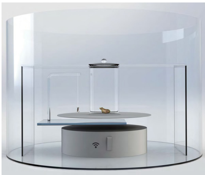
Fig. 2. The testing apparatus for both behavioral and EEG experiments. The subject was contained in a cylindrical cup made of transparent polymethyl methacrylate (PMMA), which was hung in the middle of a U-shaped frame. A rod made of transparent PMMA was bent to form a right angle and adhered onto a PMMA board that was placed on the electric turntable. A white plastic wafer was adhered to the bottom of the cup to minimize visual interference. In addition, a white opaque plastic cylinder surrounded all above components.
