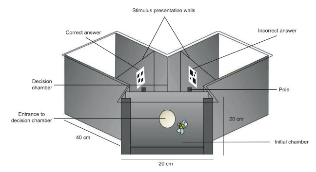
Fig. 1. Y-maze apparatus set-up for the experiments. The diagram shows parts of the Y-maze and the stimulus positions. Bees were trained to choose 4 elements when presented against the incorrect options of 1–10 (excluding 4).
