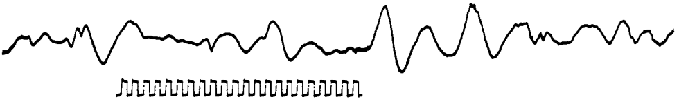
Fig. 4. Typical broad-band wave-form produced by an insect making slight movements in the web. Calibration: 50 cyc./sec.
