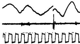
Fig. 8. Example of a 'fast transient'. Upper trace: broad band; lower trace: band-limited to 200–500 cyc./sec. Calibration: 50 cyc./sec.
