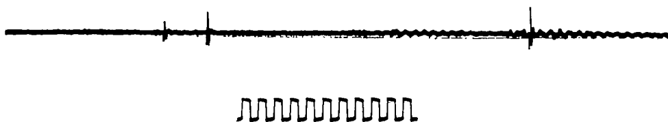
Fig. 9. Insect antenna gently drawn across the web: band limited to 200–500 cyc./sec. Calibration: 50 cyc./sec.
