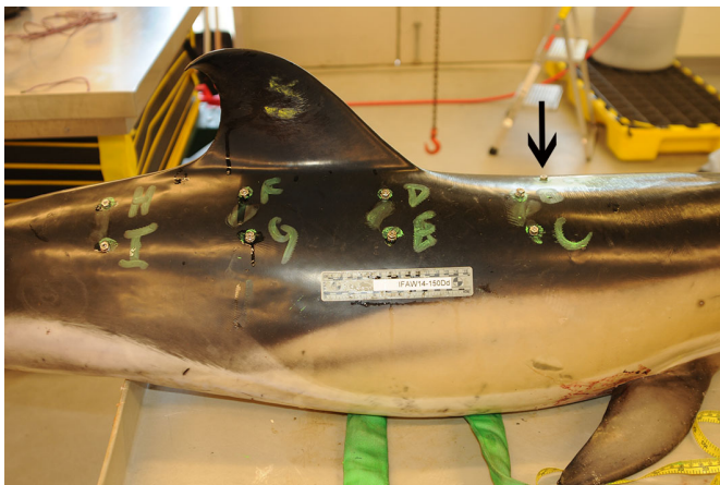
Fig. 1. Location of needle and tag insertions in dolphin cadaver blubber/muscle shearing model. Stations were labeled A through I. Station A is in the dorsal midline anterior to the dorsal fin (arrow). Stations B, D, F and H were the upper lateral line as shown in the figure, and stations C, E, G and I the lower lateral line. In this image, the scaled model tags are inserted prior to oscillation as described in the Materials and methods.
