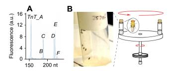
**Fig. 1. Troponin T splice variants and experimental setup.** (A) Sample trace from DNA fragment analyses of *D. melanogaster* 5' troponin T gene (*TnT*) splice variants. (B) Right, hypergravity centrifuge illustration; left, generally observed fly positions post-24 h, 12 *g* treatment, i.e. flies aligned themselves along a relatively thin strip of the outer vial wall.
