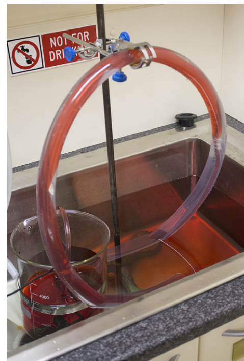
Fig. 3. Prevention of the collapse of dialysis tubing by a surrounding column of water. (A) PVC and dialysis tubing surrounded by a column of water, which protects the dialysis tubing from collapse. (B) Photograph of dyed water flowing through the dialysis tubing surrounded by a column of water in a 25 mm inner diameter (i.d.) PVC tube. The dialysis tubing was connected to 6 mm i.d. PVC tubing – the three cable ties can be seen about half-way up the right-hand side of the tube.
