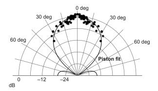
**Fig. 5. Directionality.** The directionality of calls recorded on 14 May measured in a third octave band centred on 35 kHz. The values are displayed as a mirror image to create a symmetrical plot. The black line is a fitted emission from a piston radiating sound at 35 kHz.
