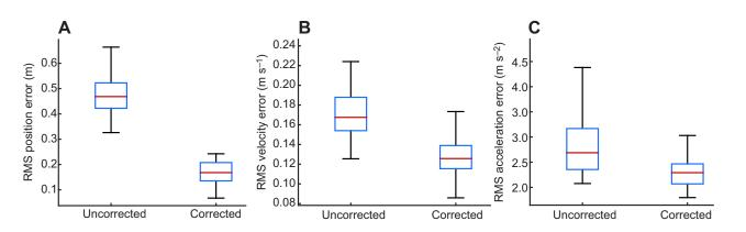
Fig. 4. The effect of oblique projection correction on the RMS errors from all 28 trials. (A) Horizontal position; (B) velocity; (C) acceleration. There was a significant difference with oblique projection correction in all cases (*P*<0.05).
