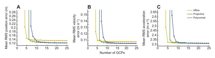
Fig. 5. The effect of different numbers of GCPs and different transformations on the mean RMS error from all 28 trials. (A) Position; (B) velocity; (C) acceleration. Affine transformation data is shown in yellow, projective in green and second-order polynomial in blue. For reasons of scaling, the minimum number of GCPs is not displayed.
