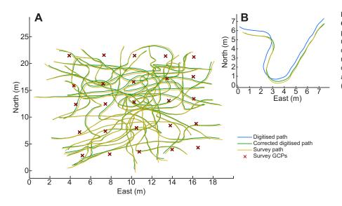
Fig. 2. Relative positions of digitised trials and GPS surveyed paths. (A) The corrected digitised paths (green) and GPS surveyed paths (yellow) relative to ground control point (GCP) locations (red crosses) for all 28 trials. (B) A typical example of the raw digitised path (blue) and the oblique projection-corrected digitised path (green), compared with the actual GPS surveyed path (yellow), from one trial (projective transformation with all 25 GCPs).
