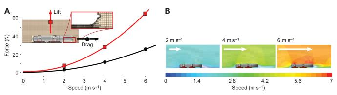
**Fig. 4. Lift and drag forces on a DTAG2 increase with speed.** (A) Lift (red) and drag (black) forces (N) on a DTAG2, and (B) flow visualization at uniform velocity profiles of 2, 4 and 6 m s<sup>-1</sup> from computational fluid dynamics (CFD) simulations using STAR-CCM+ (version 9.04) over 9.6 m cells, with extra mesh refinement in the region located under the tag (A). See main text for further CFD details.
