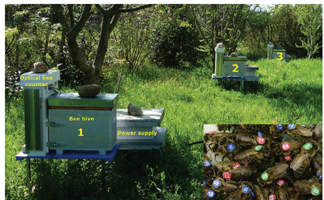
Fig. 2. Optic bee counters in the field measuring the activity of honey bees with coloured tag numbers. The optic bee counter (at the entrance of the hive) and the power supply (next to the hive) were protected from climatic events by a wood box covered with a metal top. Bees identified with coloured tag numbers are shown in the inset.
