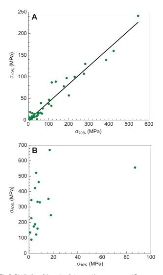
Fig. 5. Distribution of the pairs of stresses (A:  $\sigma_{10\%}$ ,  $\sigma_{20\%}$ ; and B:  $\sigma_{60\%}$ ,  $\sigma_{10\%}$ ) as obtained from tensile tests. The straight line in A is the result of a linear regression analysis. No clear correlation can be established between the values of  $\sigma_{60\%}$  and  $\sigma_{10\%}$ , consistent with the statistical analysis of independence.
