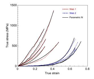
Fig. 6. Comparison of the experimental true stress( $\sigma$ )-true strain ( $\varepsilon$ ) curves (broken lines) and reconstructed stress-strain curves (solid lines) for the two different webs presented in Fig. 4.
