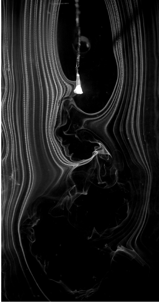
Fig. 9. Smoke visualization to the vortex wake of a 5 cm diameter cylinder at 1 \text{ m s}^{-1} . Note the secondary instabilities ('curls') in the wake.
