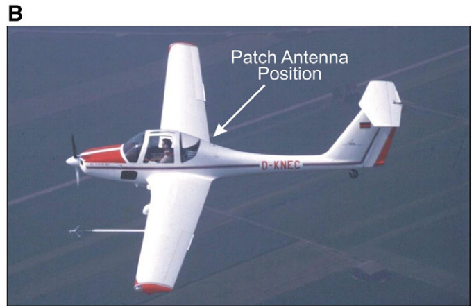
Fig. 1. GPS logger and research aircraft used in flight testing. (A) A miniaturized GPS data logger with an attached 25×25 mm patch antenna used in the albatross flight measurements is depicted. (B) The GPS logging unit, which includes the logger, the batteries, the wiring and the casing, was flight tested using several aircraft. The vehicle shown is a research aircraft of the Institute of Flight System Mechanics of the Technische Universität München.
