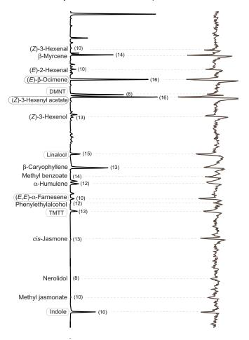
Fig. 5. Averaged gas chromatography–electroantennographic detection (GC–EAD) trace of responses from antennae of mated female *S. littoralis* moths (right-hand trace) to headspace collections of cotton plants damaged by the larvae of *S. littoralis* (left-hand trace). The number of responses to the compounds identified by gas chromatography–mass spectrometry is given on the right-hand side of the GC-trace. The circled compounds represent the seven *de novo* GC–EAD active compounds found.
