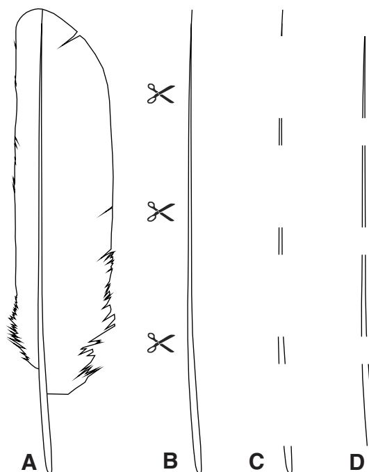
Fig. 1. Schematic drawing of the sampling of nanoindentation and bending test specimen. (A) Complete feather. (B) Feather rachis after removing the vane with scissors. (C) Specimen for nanoindentation (length: 10 mm each). (D) Specimen for two-point bending tests (length: 40 mm with the exception of the most distal part of pigeon feathers, which was 30 mm).
