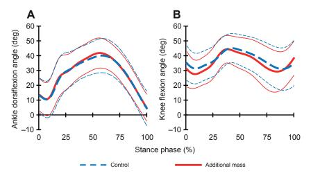
Fig. 6. Inside limb (A) ankle and (B) knee angles during stance. For the instants where the maximum joint moments were generated, no difference was observed between conditions for either the ankle or knee joint angle. The thick lines represent the average value across all the subjects and the thin lines indicate ±1 s.d.
