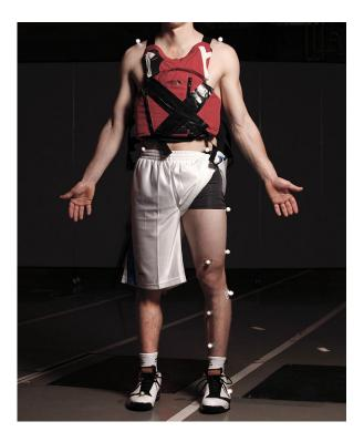
Fig. 1. Photograph of the modified lifejacket (total mass=12.4 kg; 16.5% body mass for sampled population) worn by a subject. Six pieces of diving lead were placed surrounding the bottom region of the jacket near the body center of mass.
