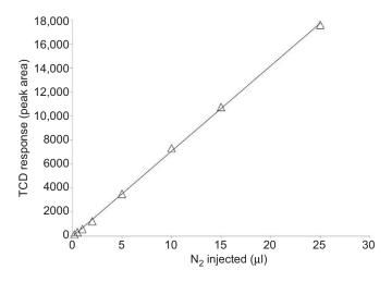
Fig. A1. Standard curve for injections of known amounts of N<sub>2</sub>. Points show the linear response of the thermal conductivity detector as a function of the amount of pure nitrogen gas injected into the gas chromatograph; the variables were highly correlated ( $R^2$ >0.99).
