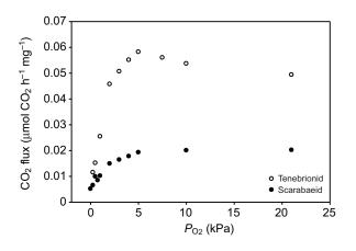
Fig. 5. Mass-corrected mean CO<sub>2</sub> release rates (averaged across species) plotted *versus*  $P_{O_2}$  for tenebrionid (filled circles) and scarabaeid (open circles) species. Scarabaeids had significantly higher CO<sub>2</sub> release rates than tenebrionids at every  $P_{O_2}$  (*P*<0.05), and  $P_{O_2}$  had a significant effect on CO<sub>2</sub> release rates across both families (*P*<0.05).
