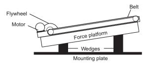
Fig. 1. Force-measuring treadmill mounted at 9 deg.
