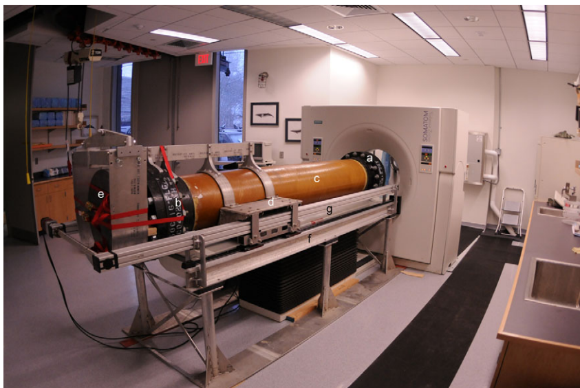
Fig. 1. Hyperbaric imaging system. The chamber consists of a fiberglass pipe with end flanges (a,b) and caps rated to 1720 kPa. A dead seal or dolphin is placed in the imaging portion (c), restrained with suction cups to the chamber wall, and the chamber filled with water. A hydraulic press allows pressurization to the desired depth equivalent. The chamber rests on a carriage (d) and it has a counterweight (e). The carriage runs on a pair of rails (f) to accommodate the loaded weight as that exceeds the scanner table capacity. The rails are motor driven via continuous belts (g) to follow the movement of the scanner table. Spiral CT scans were acquired for each subject at a series of pressures.
