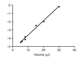
Fig. 1. Calibration curve for Millar conductance catheter placed in tubing of differing diameters filled to a depth of 6 mm with 0.8% saline. Conductance in expressed as arbitrary units.
