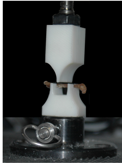
Fig. 1. Photograph of a femur loaded in a United SSTM-1 testing machine just prior to application of breaking force. The area behind the testing fixture is blacked out to enhance visibility. The fixture was designed to maximize the span, hold the bone in one position, and resist deformation during breaking. All bones were loaded in the position shown.
