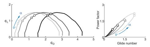
Fig. 8. Illustration of how the lift–drag polar is related to the performance polar. Decreasing minimum drag coefficient, which occurs for increasing Reynolds number, increases performance (starting with black and ending with gray we plot polars for drag coefficient at zero lift  $C_{D0}$ =1.6, 0.8, 0.4, 0.2, 0.1). A circle indicates maximum power factor and a square maximum glide number.
