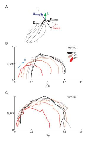
Fig. 2. Sweep does not increase the lift created by a translating fruit fly wing at Re=110 and 1400. (A) The lift ( $C_L$ )-drag ( $C_D$ ) polar shown for Re=110 (B) and Re=1400 (C) represents the dimensionless lift (L) and chordwise drag ( $D_{chord}$ ) forces obtained by varying the angle of attack ( $\alpha$ ) from 0 to 90° in steps of 4.5°. We tested this for wing sweeps from 0°, indicated with black, to 60°, indicated with red, in increments of 10° sweep.
