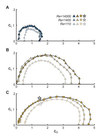
Fig. 7. Lift and drag augmentation of the LEV varies little with Reynolds number. (A) Unidirectionally translating wing. (B) Unidirectionally revolving wing. (C) Reciprocally revolving wing; star represents fruit fly kinematics. The force polars at *Re* 1400 and 14,000 overlap for angles of attack lower than  $45^{\circ}$ . The main effect of a low Reynolds number (110) is that it damps both lift and drag force.
