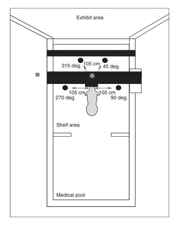
Fig.2. Testing configuration with four test speakers located 105 cm from the center of the stationing bar and 75 cm below the surface. The test speakers are represented as the black circles. The gray octagon represents the 'test trainer's' position and the gray square represents the 'data recorder's' position.
