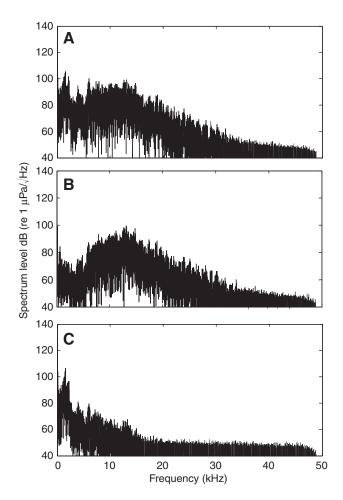
Fig. 1. Power spectra comparison of the 0.2-20 kHz (A), 6-20 kHz (B) and 0.2-2 kHz (C) broadband test signals played at the 3000 ms duration (sample rate of 97,656 Hz).
