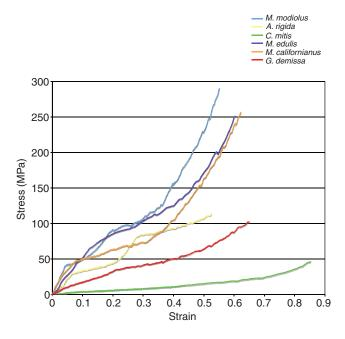
Fig. 1. Byssal thread stress–strain curves. A typical stress–strain curve was chosen for each species. Curves from a previous study have been included for comparison (Pearce and LaBarbera, 2009). Note that the *Atrina rigida* curve (yellow), like that of *Modiolus modiolus* (light blue), has two distinct yield points. The *Ctenoides mitis* curve (green) shows that these threads had extremely low strength and stiffness but were very extensible.
