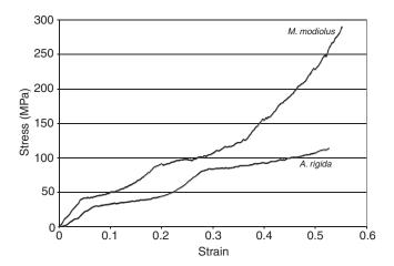
Fig. 2. Double-yield behavior. These curves illustrate the double-yield behavior of *A. rigida* and *M. modiolus* threads. Each curve has two distinct yield points, each represented by a relatively sudden drop in stiffness (the slope of the curve). Following each yield point, the thread becomes stiffer prior to either once again yielding or failing.
