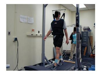
Fig. 1. Data collection procedures showing the unweighting system and weighted vest.
