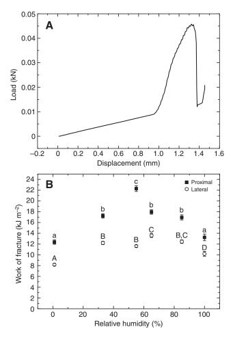
Fig. 3. (A) A typical load–displacement curve for a clipper test and (B) the work of fracture values for nail samples tested in both the proximal and lateral directions at a number of humidity levels. Groups denoted by the same character are not significantly different from each other at *P*<0.05 according to Tukey's *post-hoc* tests. Error bars are standard deviations from the mean.
