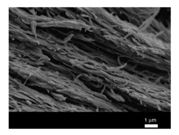
Fig. 4. Scanning electron microscope image of a torn nail sample fractured in the lateral direction.
