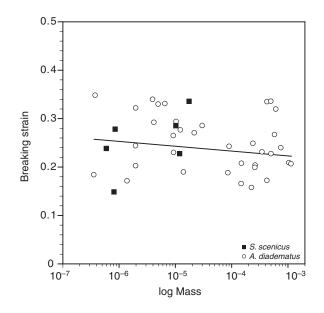
Fig. 4. Breaking strain is normally distributed (*P*=0.47), with a mean (±s.e.m.) 0.249±0.009, for combined data from both *A. diadematus* and *S. scenicus*. There is no statistically significant trend with log-transformed spider mass (*M*). The least-squares regression best-fit for the combined data was  $\varepsilon_{max}$ =0.237–0.008log*M*, *r*<sup>2</sup>=0.02, *P*=0.35.
