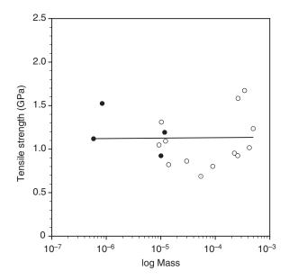
Fig. 5. Silk tensile strength ( $\sigma_{max}$ ) plotted against spider mass (*M*). There is no statistically significant trend of tensile strength with log-transformed spider mass. The least-squares regression best-fit for the combined *A*. *diadematus* and *S*. *scenicus* data sets was  $\sigma_{max} = -114 \times 10^{9} \pm 2.00 \times 10^{-6} \log M r^{2} = 0.0002$  R=0.06
