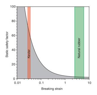
Fig. 2. The solid line shows the form of Eqn 5, which indicates the effect of breaking strain on the minimum static safety factor required for bungee jumping. The gray shaded area below the solid line represents strain–safety factor combinations that would fail during bungee jumping. For example, a strand of Kevlar would require a static safety factor of at least 58, while natural rubber would only need a static safety factor of approximately 3 to survive a bungee jump.
