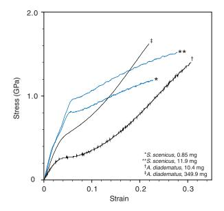
Fig. 3. Sample data from several silk tests to failure from juvenile and adult spiders. *Salticus scenicus* are shown in blue and *Araneus diadematus* in black. Note the difference in shape of the stress–strain curves for the two species.
