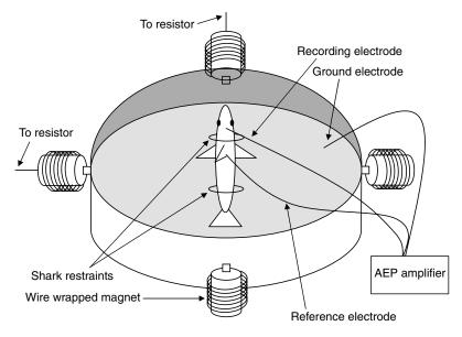
Fig. 1. Diagram of the directional shaker table setup. The fifth, mechanical shaker, which produces the up/down motion (*Z*-axis) of the dish, is located under the dish and not visible in this picture. Drawing not to scale.
