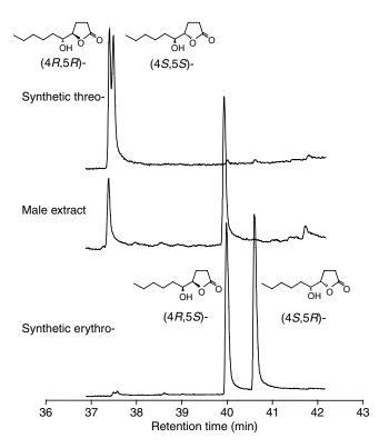
Fig. 2. Separation of synthetic threo- and erythro-enantiomers of 5hydroxy-4-decanolide (HDL) on a chiral  $\beta$ -DEX 225 GC column. Extracts from *N. vitripennis* males contained (4*R*,5*R*)- and (4*R*,5*S*)-HDL.
