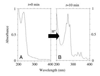
Fig. 3. Effect of acidification on BMSF. Product was collected from initial RP-HPLC separation at pH 7.0 (A), the pH was adjusted to 3.5 using acetic acid and the changes in UV absorbtion monitored spectrophotometrically at RT (B).
