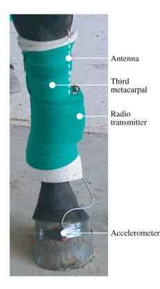
Fig. 2. Hoof-mounted accelerometer and telemetry unit, antenna and battery mounted in an elasticated exercise bandage on the lateral aspect of the third metacarpal bone.
