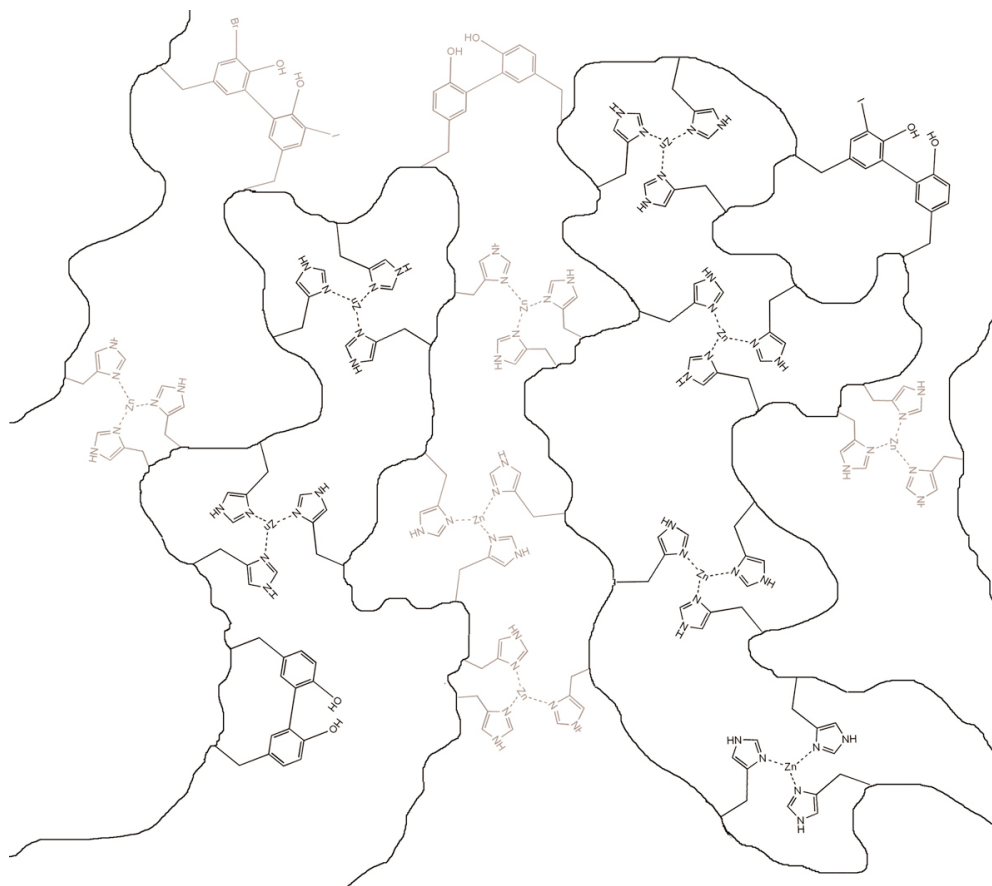
Fig. 7. Schematic of proposed cross-linking in Nereis jaws. Zn-mediated cross-linking of histidine-rich proteins is proposed to be responsible for enhanced hardness and modulus in Nereis jaws. Cross-linking may be intramolecular (black complexes) or intermolecular (grey complexes). Additional cross-linking via di- and/or tri-tyrosine formation is not expected to contribute significantly to mechanical properties of the bulk jaw.
