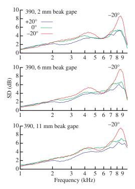
Fig. 10. Acoustic output became more directional when the microphone was lowered  $20^{\circ}$  but became less directional when the microphone was elevated  $20^{\circ}$ . Directionality (s.D.) was calculated as in Fig. 9.
