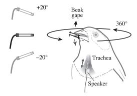
Fig. 2. Illustration showing where a small speaker was inserted into the trachea, how beak gape was varied, and how subjects were rotated with respect to microphone positions. Beak gape was measured as the distance between the tips of maxilla and mandible.
