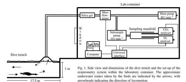
automatically corrected the measured flow to STPD (273 K and 101.3 kPa). A sub-sample of  $10\,l\,\text{min}^{-1}$  was bled into a manifold from which an oxygen (paramagnetic O<sub>2</sub>-analyser PA-1B; Sable Systems; resolution, 0.0001%) and CO<sub>2</sub> analyser (Beckman LB2 Medical CO<sub>2</sub>-analyser, Schiller Park, IL, USA; resolution, 0.01%) sampled in parallel. All connections between the various components of the respirometry system were made with gas-impermeable Tygon tubing.
