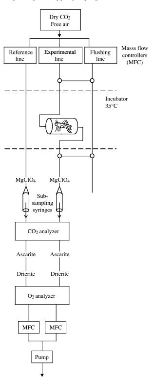
Fig. 1. Schematic of the respirometry set-up.
