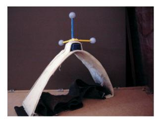
Fig. 2. The harness employed for attachment of the inertial sensor to the thoracic spinous processes of the subject animal. The wands and markers for 3D optical motion capture are also shown.
