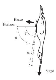
Fig. 1. Attachment of data-logger on bird's back. Diagram shows angle of Y (surge) axis of logger to horizon ( $\gamma$ ), that of body axis to horizon ( $\theta$ ) defined as body angle (negative as the bird descends) and logger attachment angle ( $\alpha$ ).
